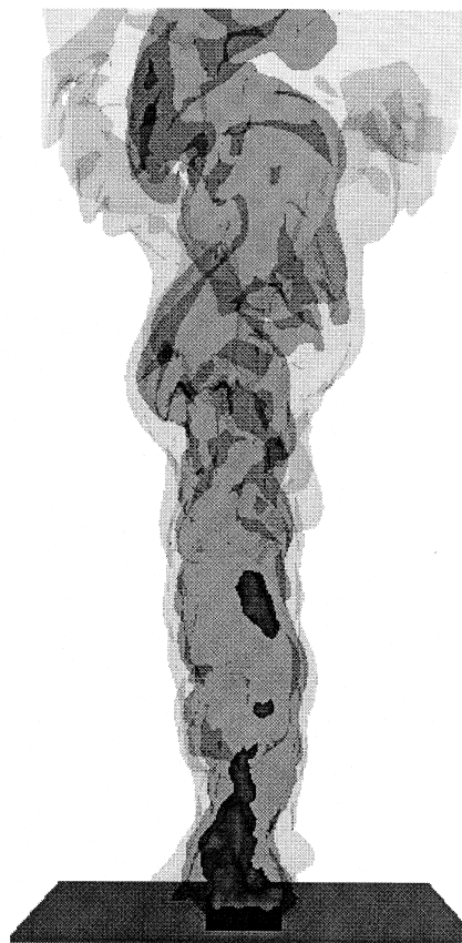
Figure 1 Instantaneous snapshot of a pool fire simulation performed on a 96 \times 96 \times 96 grid. The contours correspond roughly to the boundaries of the continuous flame, intermittent region, and plume. The square burner is of length D^* with the height of the computational domain rising to about 12 D^* .
